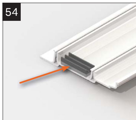
54 Fit the internal fascia claddings to the eaves beam, ensure the fascia corner packers are attached on the inside of the fascia at each corner.
