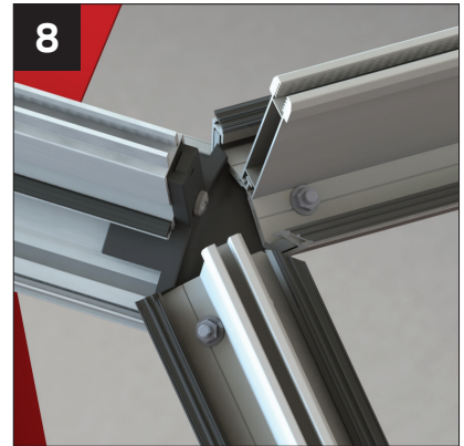
8 Using nuts and bolts provided, locate each hip bar and secure to radius end by hand tightening nuts.
